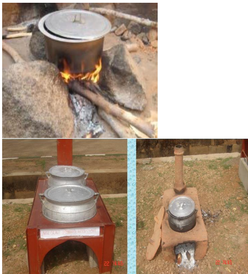
Fig. 5: The Traditional Three-Stone Cooking Stove and Highly Improved Wood Saving Stoves
